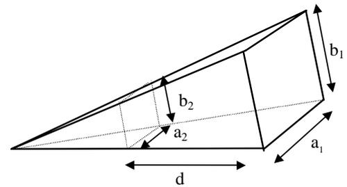
Figure 2: Geometry of tapered resonant cavity in GTEM
