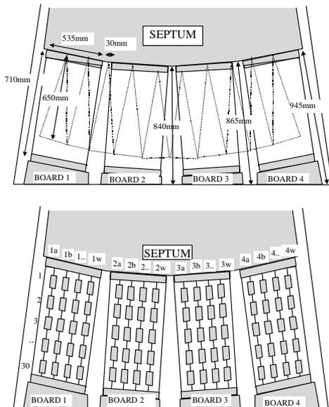
Figure 4: Resistor boards (plan view)
