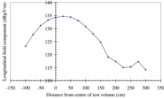
Graph 2: Variation of longitudinal field component along the axis of the cell, 1W input power.
