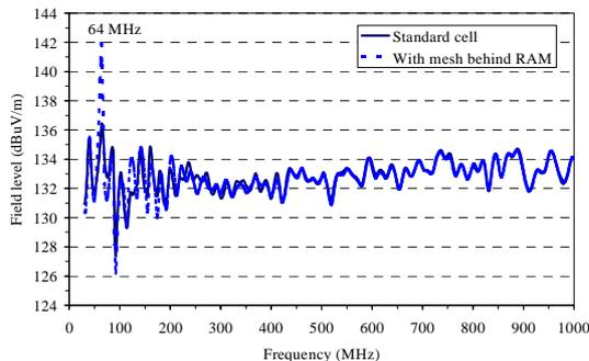
Graph 9: Effect of mesh behind RAM on vertical field component of GTEM 1750.
