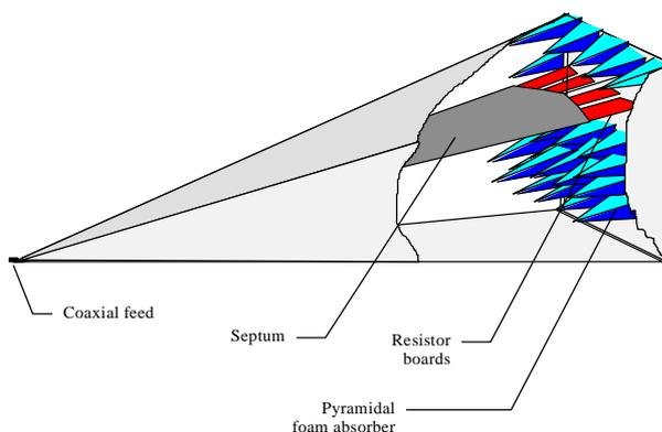
Figure 1: Schematic diagram of the GTEM cell.
