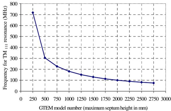
Graph 5: Frequency of TM<sub>111</sub> mode resonance for different sizes of GTEM cell.
