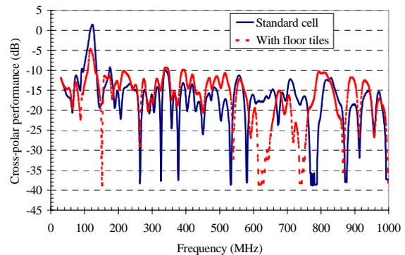
Graph 11: Effect of ferrite tiles on cross-polar performance of GTEM 1750.
