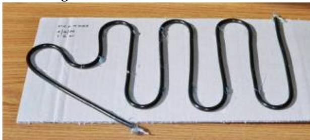
**Figure 3** The test meander cable.
