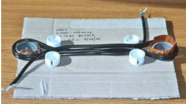
**Figure 10** The second method of damping is to add *resistively-loaded* loops closely coupled to the cable loops.
