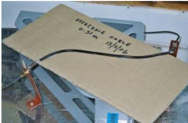
**Figure 2** In the test set-up the VNA reference planes are at the connectors on copper strip brackets.
