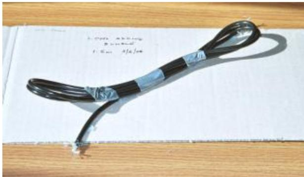
**Figure 5** A “traditional bundle” wound with the end loops inductively *adding*.
