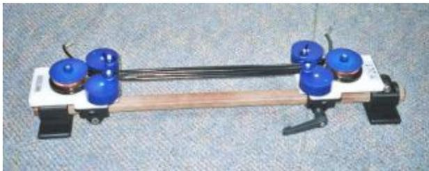
**Figure 12** A “practical” version of the resistively-loaded opposed-loop bundle.
