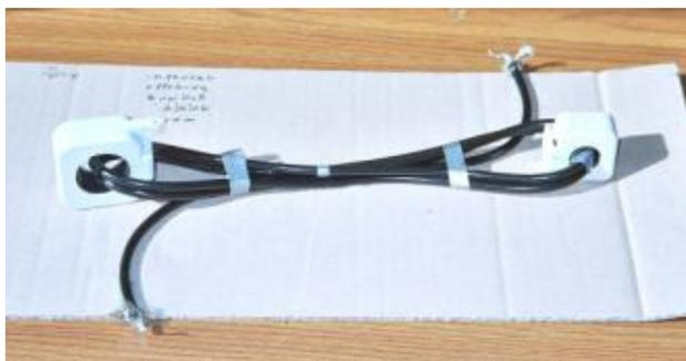
**Figure 8** A ferrite ring may be clipped over each end loop-pair of the bundle of Figure 5.
